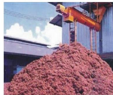
**Gambar 3.** Serabut (Fiber) Kelapa Sawit
